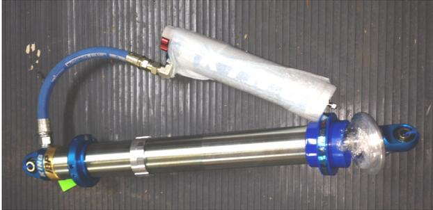
New 2.5 king coil over shocks, 14" stroke shock, remote reservoir with compression adjustment clickers and internal triple bypass, part # RS2514- COHRS coils are available as well. \$630 each
